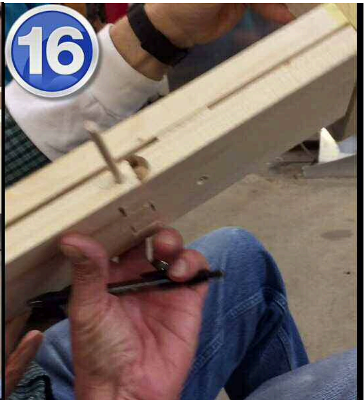
Leg cut out to allow entire wooden hinge to lay flat against the table base
